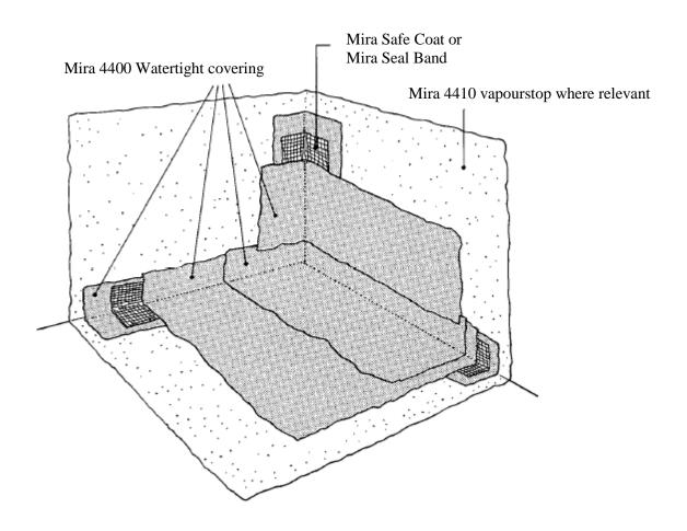
Note. When the Mira 4500 Vapour mat is required, it is installed between the two layers of Mira 4400 Mira Multicoat.
